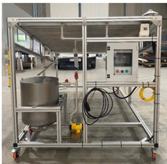
Figure 11: Rear view of the reactor, indicating how to turn on the pump
