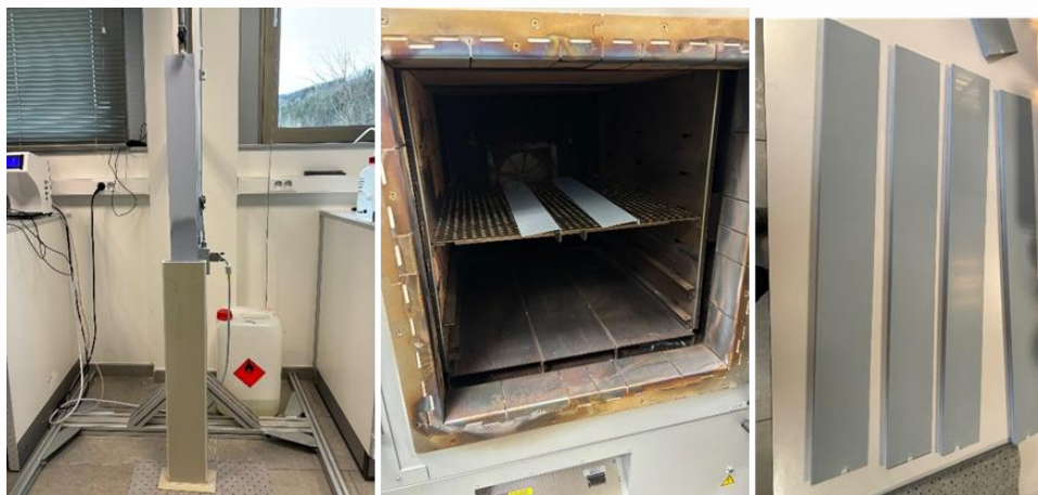
Figure 20: TEOS/ \text{TiO}_2 coatings in stainless-steel preparation procedure at TEKNIKER
