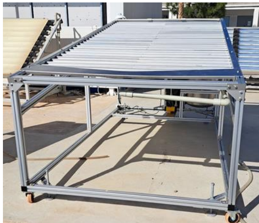
Figure 22: Immobilized TiO 2 onto the stainless-steel staircase of the ENERGICA MSCR at CIEMAT-PSA facilities
