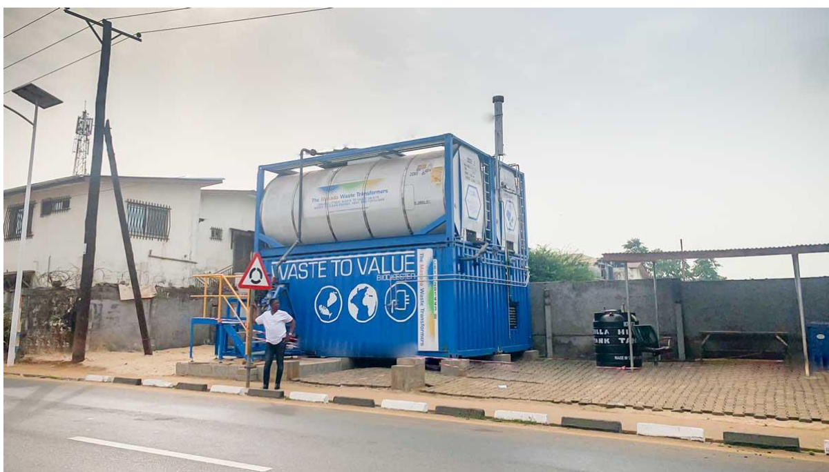
Figure 3 - A Waste Transformer V2 as implemented in Sierra Leone at the Aberdeen Woman's Centre
