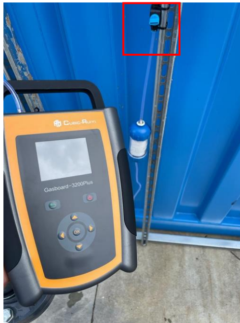
Figure 1. Biogas analyser (Cubic-Ruiyi Gasboard-3200Plus) connected to sampling point when manual valve is closed
