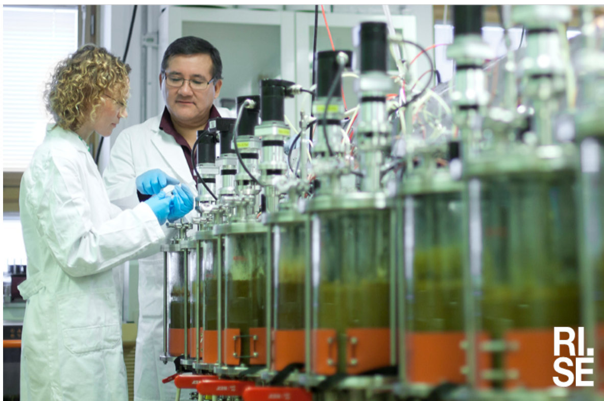
Figure 7. Continuously fed 10 L laboratory scale complete mix anaerobic reactors in the RISE biogas laboratory.
