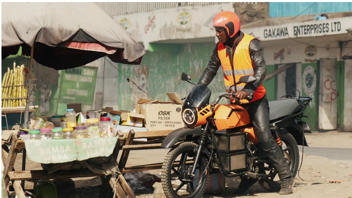
Photo of the Roam Air motorcycle, note the two rectangular removable batteries located behind the front wheel and below the rider.
